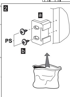
**Note:** Screws for connecting top plastic part should not be screwed very hard, because of moving the plastic part easily left or right side.
