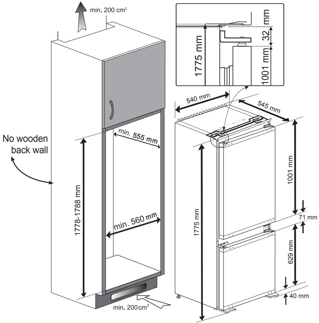
The back wall of the wooden cabinet must be left open completely to kitchen wall in order to allow sufficient air circulation to cool down the condenser unit for energy efficiency.
